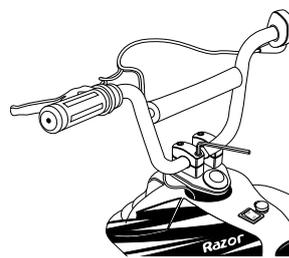
**3** Insert bolts and tighten securely. When properly tightened, the handlebars should not move forward or back.
