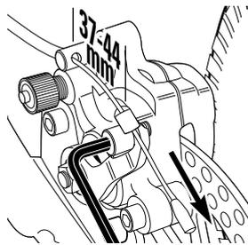
**2** Locate the rear brake caliper and disk brake behind the right rear wheel. The distance of the brake wire between the end of the cable and the anchor bolt should be between 37 and 44 mm. If the rear brake has too much slack, loosen the rear anchor bolt with a 5mm key wrench and pull the brake wire tighter (direction indicated with arrow).
