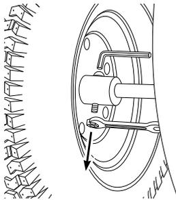
**2** Remove the bolt on the inside of the rear wheel. Remove nut and pull bolt out of axle.
