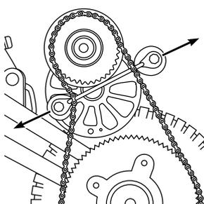
**5** Spread the chain tensioner apart to loosen chain.
