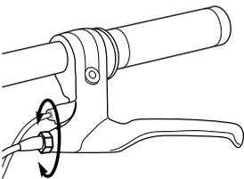
**1** To adjust the play, thread the brake lever adjuster in or out 1/4 to 1/2 turn until the desired brake adjustment is attained. Most adjustments are complete at this step. If brake still needs further adjustment, proceed to step 2 for rear brake.
