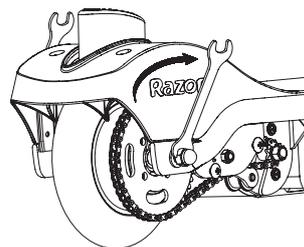
**6** With two 13mm open wrenches, re-tighten the locknuts.
