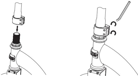
**1** Loosen the collar clamp and slide it upward. With a clock-wise twisting motion, push and “thread” the steering tube onto the fork until it bottoms out on the fork headset lock nut.
