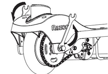
**2** Using two 13mm open wrenches, loosen the locknuts by turning the wrenches counter clockwise.
