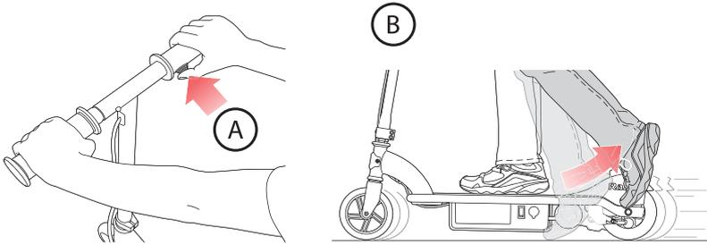
To start unit, turn on power switch, press the push button throttle (A) and kick start up to 3mph (5mh) (B).
