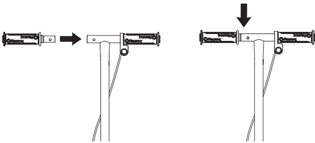
**1** Insert and secure the collapsible handlebar by pressing the spring-loaded button and inserting it into the T-bar.
