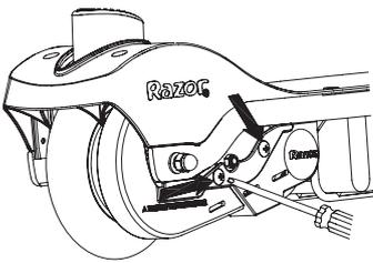
**1** With a Phillips screwdriver, loosen the two screws and remove the chain guard.
