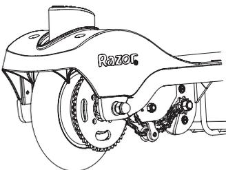
**4** Remove wheel and install replacement wheel. (Note the sequence of the hardware)
