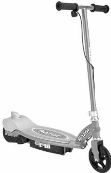
**⚠ NOTE:** The unit must be traveling up to 3mph (5kmh) before motor will engage. Kick start up to 3mph (5kmh) while applying the throttle to engage motor.
