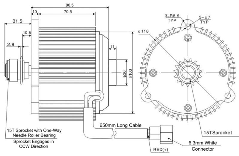
This motor can only be used with its shaft spinning counterclockwise. If wired to spin clockwise the sprocket will not engage.
