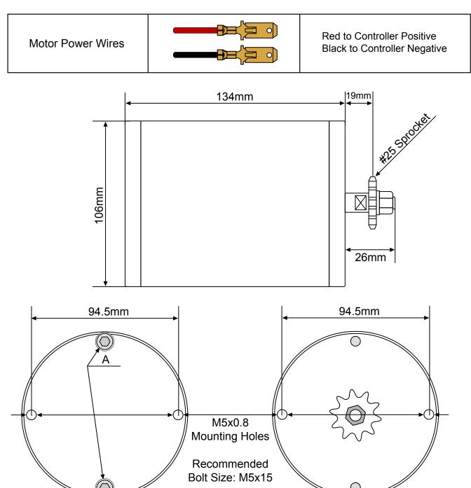
A = Recessed motor assembly bolts provide a flat backplate with no bolt heads protruding out of it.
