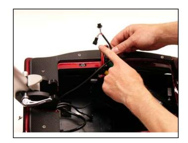
10. Installation is the reverse of the removal procedure. Note that there is an individual small plug with a red, brown and black color code that does not conect to any thing on the controller. This plug is not used on the SX 600.
