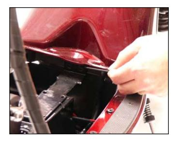
4. Remove the two rear bolts with a 3mm allen wrench.
