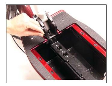
3. Remove the two front bolts with a 3mm allen wrench.
