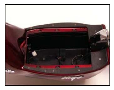
9. Completely Remove the controller.
