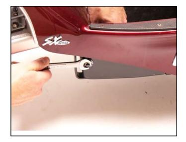
8. Unscrew the nut holding the circuit breaker in place and remove the circuit breaker.
