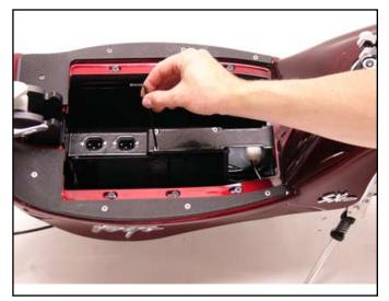
2. Remove the four to six top screws with a 2.5 mm allen wrench.
