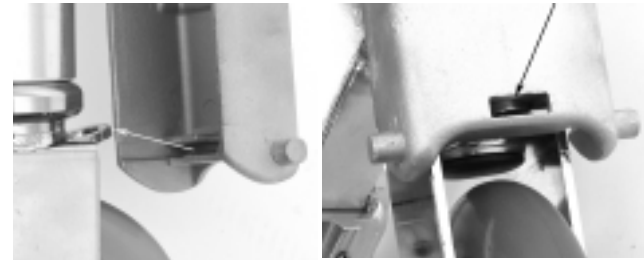
Aligning the fork to the bracket
