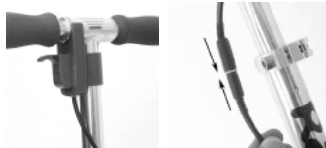
Final connection of the wiring (right)
