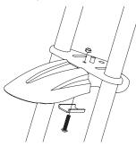
**1** Align fender with the hole in the fork and insert the bolt. Tighten securely using a 10 mm wrench and 5 mm Allen wrench.
