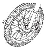
MX500/MX650 Models **3** With a 14 mm and 17 mm wrench, tighten the front wheel.
