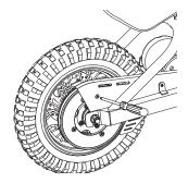
**1** Loosen screws and remove chain guard.
