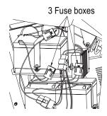
1 Remove the seat fairing and battery cover to locate the 3 fuse boxes attached to the batteries.
