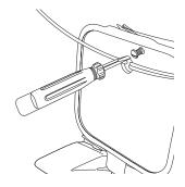
**MX500/MX650 Models** Remove screw from front fork. Align the number plate with the hole in the fork and tighten with a Phillips screwdriver.
