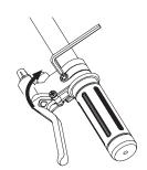
**3** Adjust the brake lever adjuster to the proper place and tighten it with the 5 mm Allen wrench.
