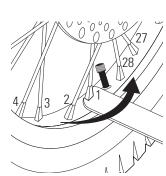
**2** Start with spoke closest to the tire valve stem and tighten each nipple, in sequence, exactly 1/4 to 1/2 turn. A single 1/4 to 1/2 turn may not be enough to bring the spokes into proper tension. Continue tightening all spokes, no more than 1/2 turn, in sequence until all spokes are tight.
