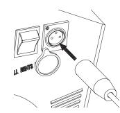
**2** Maker sure power switch is in the **OFF** position. Plug the charger into the charger port. The light on the charger should turn red during charging then back to green when charging is complete. **WARNING:** Use ONLY with the recommended charger. Batteries are only to be charged under adult supervision. The charger is not a toy. Always disconnect the charger before wiping down and/or cleaning the motor bike with a damp cloth.
