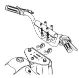
**1** Place the handlebars in the handlebar clamps with tools and manual.
