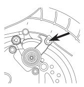
2 If the brake has too much slack, loosen the rear anchor bolt with a 5 mm Allen wrench and pull the brake wire tighter. The distance of the brake wire between the end of the cable and the anchor bolt should be between 37 mm and 44 mm.
