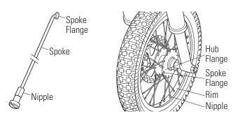
**1** Verify the spoke tension by shaking each spoke with your fingers. Spoke should not be loose from hub. Look for any play between where the spoke flanges attach to the hub. Try to turn the nipple using your fingers. You should not be able to spin any nipple by hand. If one or more spokes is loose, all spokes must be checked and need to be tightened with a spoke wrench.
