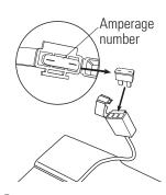
**2** Check all 3 fuses to see if the fuse(s) have burnt out. Remove any fuse that is damaged or burnt out and replace with a new one of equal amperage.
