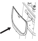
**SX500 Model** Slip the cables through the slit on the top of the number plate. Align the number plate with the holes on the fork and snap on the number plate.
