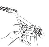
**2** Align parallel to the fork and tighten the bolts using a 6 mm Allen wrench. When properly tightened, the handlebars should not move forward or backward.
