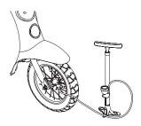
Using a bicycle tire pump equipped for a Schrader valve, inflate the tires to the PSI indicated on the sidewall of the tires.
