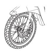
**3** Re-insert the tab on the lock washers into the holes on the front fork and tighten the locknuts on both sides of the wheel.
