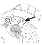
**2** If the brake has too much slack, loosen the rear anchor bolt with a 5 mm Allen wrench and pull the brake wire tighter. The distance of the brake wire between the end of the cable and the anchor bolt should be between 37 mm and 44 mm.
