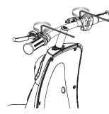
1 Loosen the 5 mm bolt located on the brake levers to adjust the angle of the brake levers to a comfortable position for the rider.
