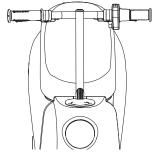
**3** Facing the front of the Pocket Mod Bellezza, position the handlebars so the throttle is on your right (the red "SAFETY ZONE" print will be facing you). Align wedge inside handlebar tube.
