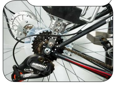
Bolt the rack's arms to the seat stay brackets (1), or to bike's seat stay mounting holes if available (2)
