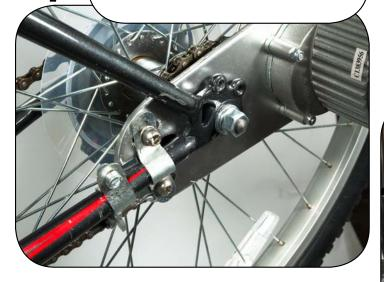
Bend-to-fit and install the two seat stay mounting brackets. This step is only necessary on bikes without pre-drilled mounting holes
