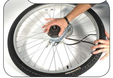
Remove the wheel's tire, tube, freewheel, and spoke protector
