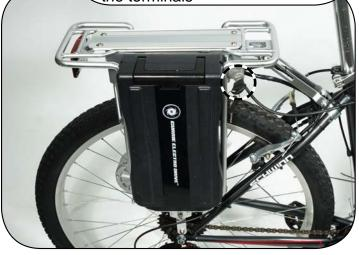
Charge the battery (8 hours initially, then 6-8 hours after each ride). The battery can be charged on or off the bike
