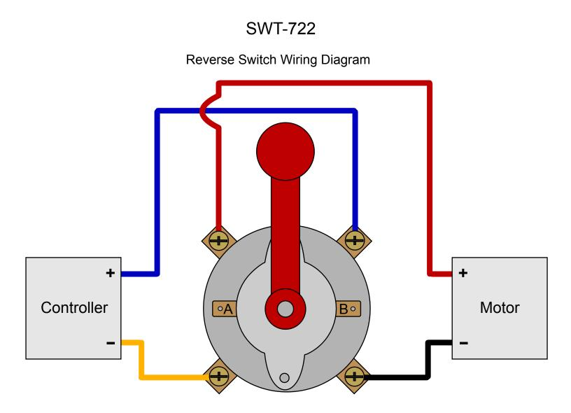
Terminals A and B are for a reverse light or buzzer and close when the switch is in reverse.
