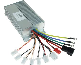
Operating Voltage: 60 Volts DC (Works with 60 Volt Battery Packs) Power: 2000 Watts (Works with 1800-2000 Watt Brushless DC Motors) Current Limit: 40 Amps (40 Amps Maximum Current Output) Low Voltage Protection: 52 Volts Works with Sensored Brushless DC Motors with 120 Degree Phases
