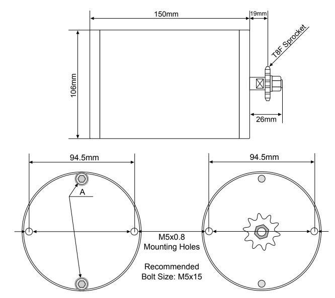
A = Recessed motor assembly bolts provide a flat backplate with no bolt heads protruding out of it.
